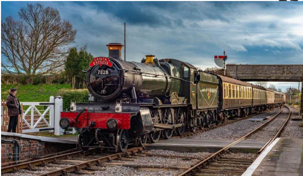
Santa Express entering Williton, hauled by BR(W) 4-6-0 Manor Class 7828 Odney Manor. Photo: Mike Lanning
