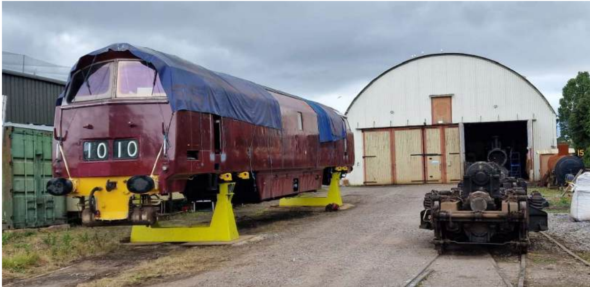
The body of Class 52 D1010 'WESTERN CAMPAIGNER' is now resting safely on the ex-BR-Swindon stands at Williton. One of the bogies can be seen alongside, before being moved the short distance to the DEPG loco shed. Pictured on Monday 8 th July 2024 by Natalie Royal ©
